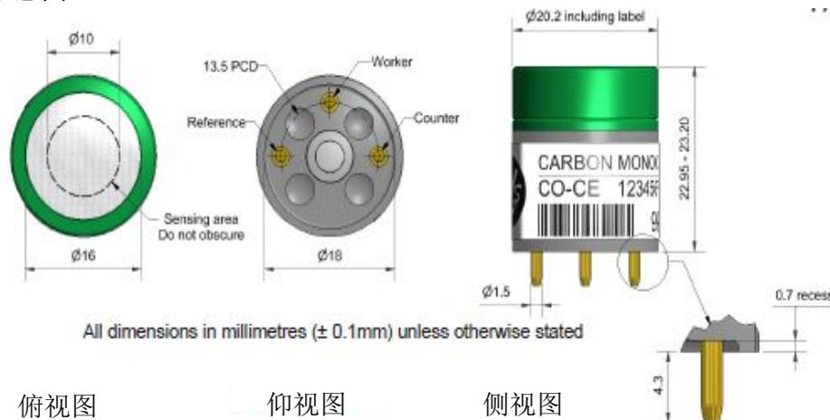
All dimensions in millimetres ( $\pm 0.1\text{mm}$ ) unless otherwise stated
